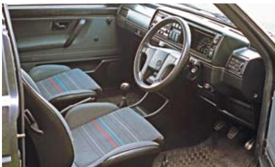
The driver's seat bolsters, particularly the one close to the door, can often be beyond repair.
